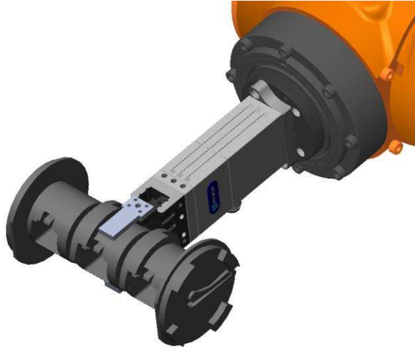
Figure 47. How the axle is gripped
