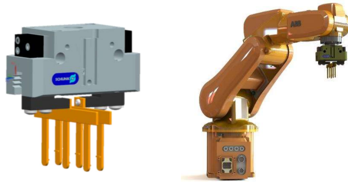
Figure 34. Gripper and fingers (left) attached to the robot (right)
